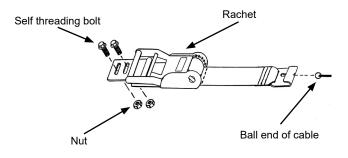
**NOTE:** Cable routing should appear as shown.
