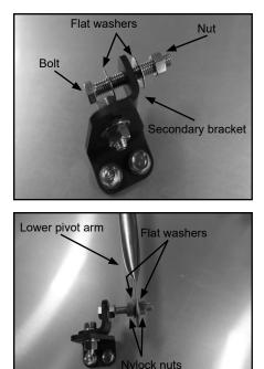
D. Thread nylock nut on hex bolt and place flat washer on bolt. Place lower pivot arm on hex bolt and secure with flat washer and nylock nut.
