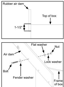
C. With rubber air dam secured, trim ends of rubber flush with front of box. If box has chamfered or radius corners, trim at start of chamfer or radius.
