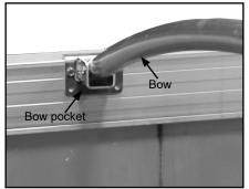
D. Place bow extension into opposite bow pocket. Secure with carriage bolt and nylock flange nut, leaving finger tight. Hold bow up to bow extension and make mark at bow extension collar on bow. Remove bow from bow pocket, then cut at mark.
