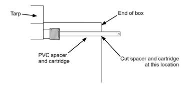
B. Measure in 1/2" from cut end and drill pilot hole, then drill 5/16" hole through PVC spacer and cartridge.
