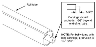
VIEW OF CARTRIDGE WHEN INSIDE ROLL TUBE
