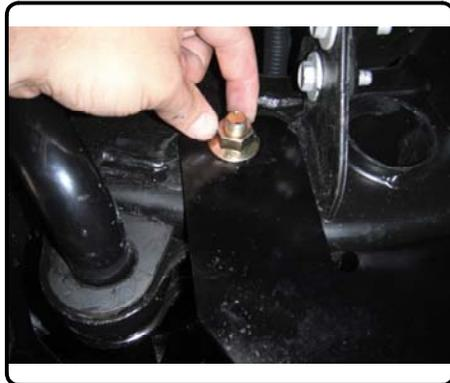
5. Torque all 1/2" fasteners to 110 lb-ft and all 12mm fasteners to 92 lb-ft.
