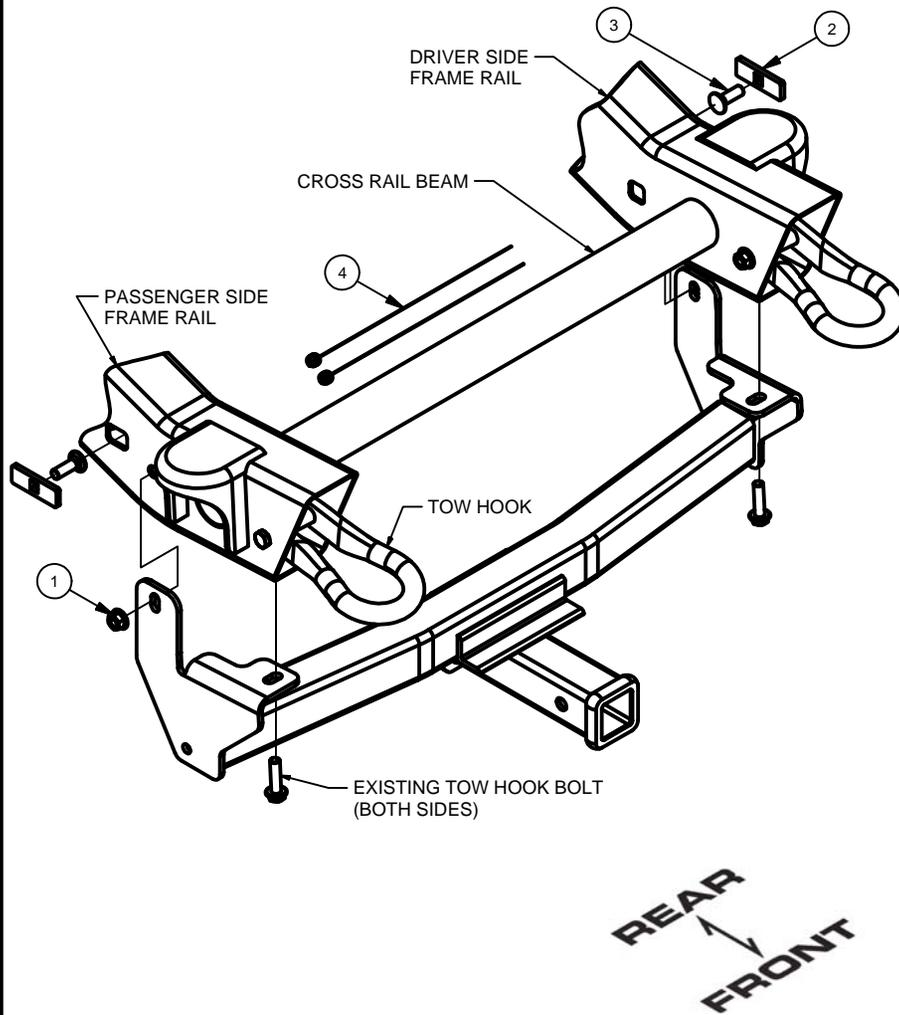
1. Using an 18mm socket, remove the (1) bolt from the bottom of the truck frame attaching the tow hook to the vehicle. Loosening the remaining tow-hook mounting bolt may be required. Repeat for other side and retain for hitch installation.
