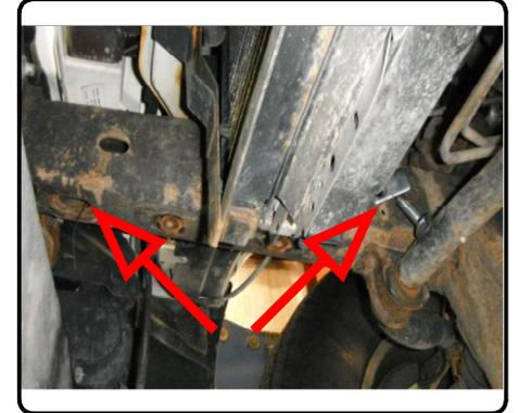
6. Raise hitch into position and secure to vehicle with 1/2" flange nuts. Torque all 1/2" hardware to 110 ft-lbs.
