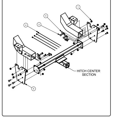
1. Use 18mm socket and ratchet to remove driver and passenger side tie down brackets if present. Existing bolt plates will fall out of front of frame rails.
