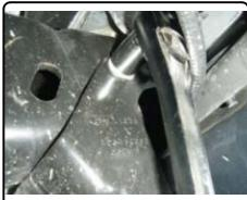
2. Return fascia brackets to vehicle owner. Fishwire the (2) remaining bolt plates through original holes on outside of frame rails. NOTE: If bolt plates are not present, use additionally supplied fasteners.
