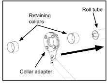
E. Center collar adapter between existing holes from removing original retaining collars, then secure retaining collars with screws using existing holes.
