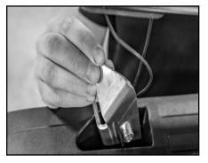
C. Move cord until pocket bracket lines up with stake pocket. Pull cord tight and place side rail on bed rail.
