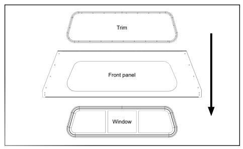
B. Secure (4) self-piercing hex screws with washers starting at corner screw locations. Adjust as necessary, then secure remaining self-piercing hex screws with washers.
